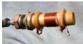
Adjustable air-wound inductor
